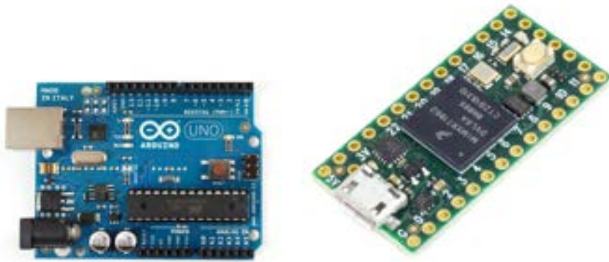
Figure 21: Arduino Uno (left) and Teensy 4.0 (right) micro-controllers
