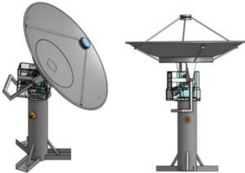
Figure 5: Design of the structure of the SRT, done by Audrey Piccini of the Structure Pole
